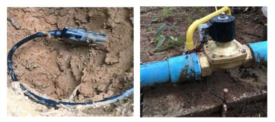
Sensors Measure Humidity, Temperature, Fertilizer (N-P-K) In the Soil, and Solenoid Valves to Control Turning the Water on and Off
